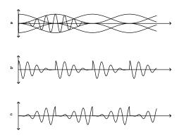
**Figure 4**. Formant generation: (a) a format as an overlapped sum of wave packets; (b, c) decomposition of the sum into realizable parts.
