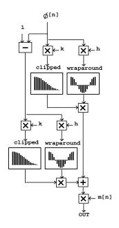
**Figure 5**. Block diagram for computing series of wave packets as shown in Figure 4.
