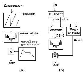
**Figure 1**. A MUSIC N instrument: (a) classically implemented; (b) adapted to use an incoming sound's phase and amplitude
