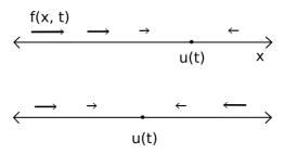
**Figure 1.** Low-pass filter considered as a dynamical system. The input, u(t), varies with time, and as a result the vector field that defines the dynamical system does also. The vector field also depends on the roll-off frequency of the filter.
