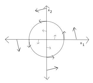
**Figure 2.** A sinusoidal oscillator realized as a two-dimensional dynamical system. The circular path is the limit cycle of the oscillator. Points that do not lie on the circle (except the origin) spiral inward or outward to the limit cycle.
