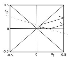
**Figure 6.** A Soft-synchronized oscillator pair as a dynamical system whose phase space is a torus. The dotted line shows the path through phase space and the solid line shows the corresponding path through one of the triangles.
