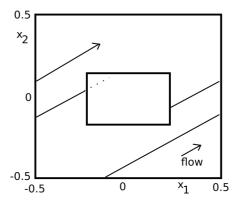
Figure 5. A phase space with a rectangular wormhole in the shape of a rectangle. The vector field is uniform, but whenever the state would enter the wormhole, instead it jumps to the diametrically opposite point.
